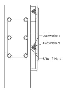
Figure 10 Attaching the Adapter Plate
